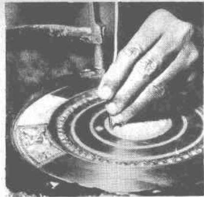
A craftsman of Tanjore, India, securing an encrusted silver ornamental medallion on a brass plate in the "nages" or "swami" process of metal decoration.
