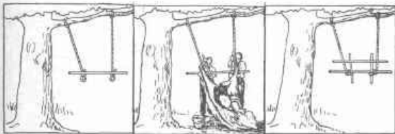
FIG. 16. Homemade beef hoist. A simple method of hoisting a beef carcass is illustrated in these sketches. A fork or rake handle or gas pipe is slipped through incisions between tendon and shank bone; ropes are suspended from tree limb or other support (wide apart at top) to height of hocks below. To free ends of rope are tied short sticks, as 2-foot pieces of broom handle or equally strong material. These are placed inside the shanks and are used as levers for winding up ropes around fork or rake handle, as shown. Two men wind up the rope around pipe or handle. When beef is at right height, another pipe or handle is laid across between ropes and ends of sticks to prevent unwinding. As the beef is raised the legs are spread farther and farther, as desired.
