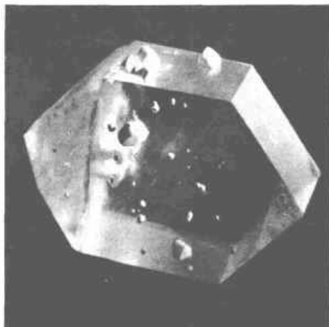
Plate 11. An ethylene diamine tartrate crystal with unexpecting crystals growing on its surfaces. Later they were identified as crystals of the monohydrate.
