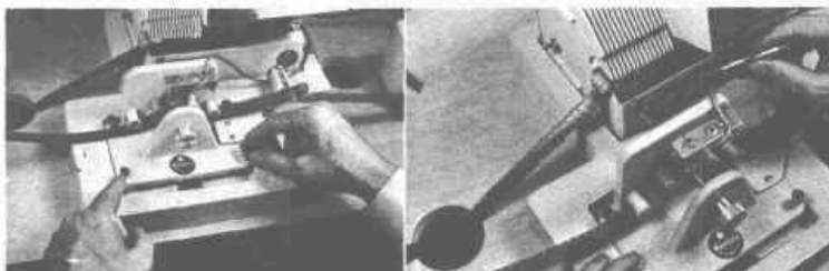
(LEFT) The Handiola is a device for achieving instantaneous positive interlock sync. Once picture and track start-marks are aligned in their respective units, sync is maintained by simply sliding tape transport assembly 1/4-inch toward viewer. Shaft engages the viewer's sprocket for positive interlock between both media, running forward or backward; movement of either medium causes the other to move in sync. Note inching knob on front of tape transport, for precise cuing without handling tape or film. Accessory frame counter is shown installed at right. (RIGHT) Pen points to interlock shaft, at point of connection with viewer, 1/4-inch movement of tape assembly establishes and releases interlock.
