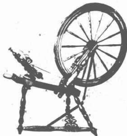
The flyer wheel. (A) stock (B) legs (C) treadle (D) pitman (E) drive wheel (F) drive wheel posts (G) drive band (H) flyer assembly (I) tension adjustment.
