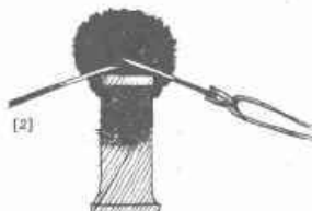
Welding: [1] where to place blows for a lap weld, [2] how to hold iron on anvil before the first blow.
