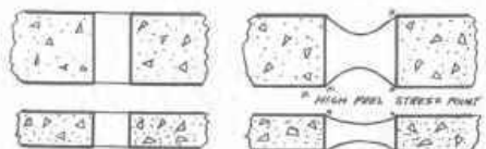
FIG. 10-4. Effect of joint shape on necking.
