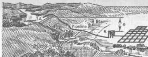
FIGURE 39. Water-supply pipeline. Practically all of the difference, h , in level between A and B represents energy expended by the water in overcoming pipe-flow resistance.
